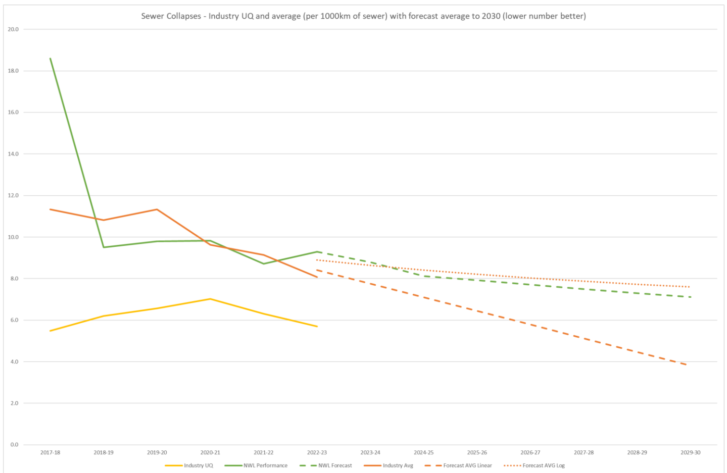
FIGURE 112: FORECASTING FUTURE SEWER COLLAPSE PERFORMANCE USING HISTORIC INDUSTRY TRENDS.
