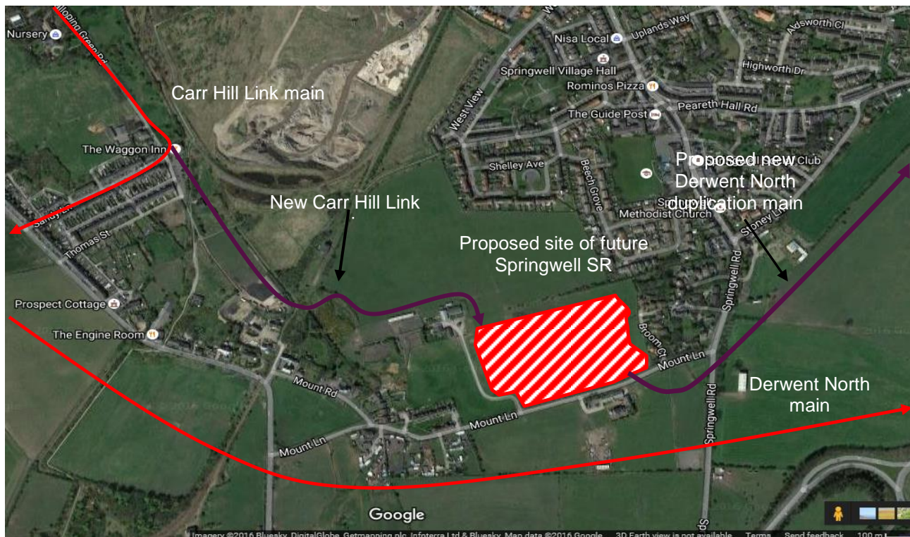
Figure 27 – schematic of proposed service reservoir at Mount Lane, Springwell Village Gateshead.
