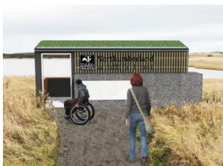
Computer image of one of the new hide renovations which include a wider more level path, wider doorway and lower, wider viewing points for those in wheelchairs
